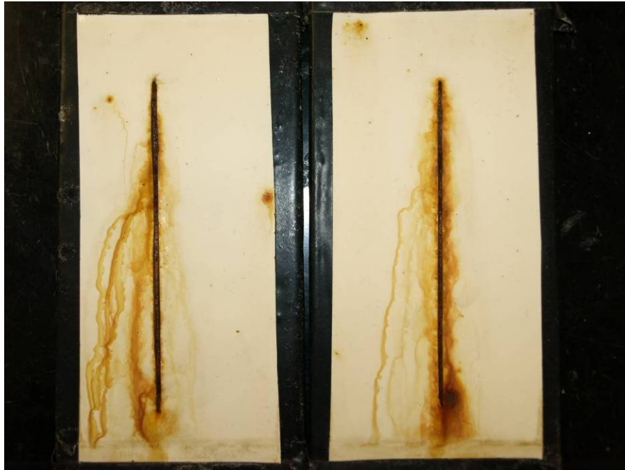
KTA-3 and KTA-4 Following 1500 Hours Exposure to Cyclic Weathering
