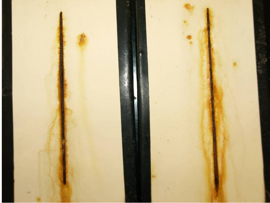
KTA-1 and KTA-2 Following 1500 Hours Exposure to Cyclic Weathering
